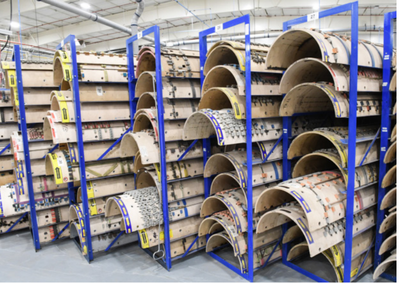
Racks hold numerous "tools" used to imprint ink graphics and text onto boxes.
